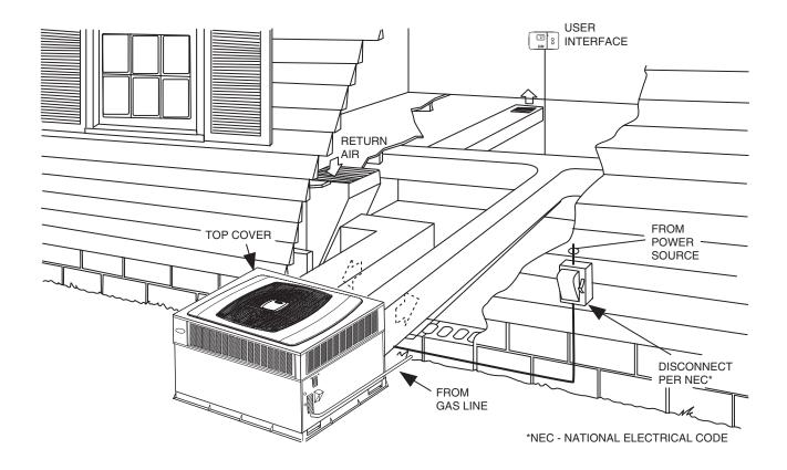
Fig. 10 - Typical Installation
